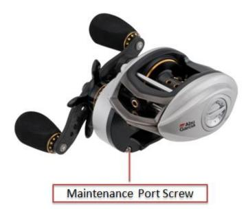
Using a small philips head screwdriver, rotate the screw counterclockwise until free. The small "door" can now be removed. Lightly grease the exposed main gear with a quality grease such as <u>Abu Garcia Precision Grease</u>. Once maintenance has been completed, reposition the door over the maintenance port and reinstall the maintenance port screw. Tighten the screw with a philips head screwdriver by rotating it clockwise. Do not over tighten.
